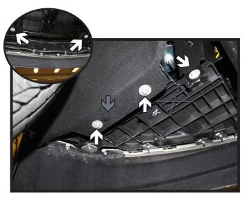
4. Using a 10MM socket, remove the eight (8) screws from the underside of the fascia. There are three (3) on each side and two (2) in the middle. Remove the two (2) push pins located in front of the tires (gray).
