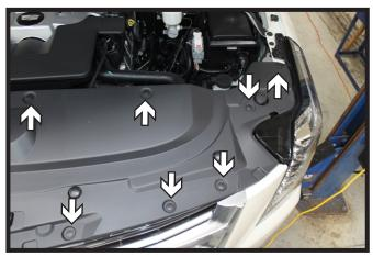
1. Remove the fourteen (14) push pins from the fascia cover and set aside. There are seven (7) on each side.
